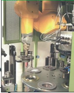
6-axis robot used for assembly and press tool loading. Stäubi approved integrator Conveyor system with component wash
