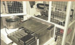
Typical loading system for a machine tool or machining centre
