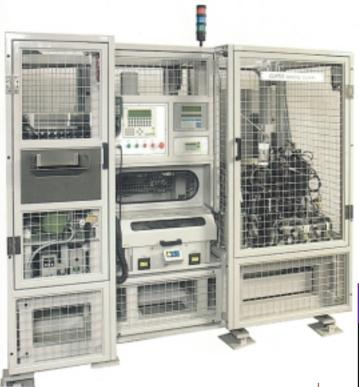
System incorporates machine loading, component measurement, deburring, washing, assembly, functional testing, disassembly and return to pallet
